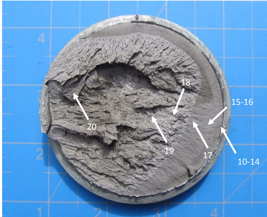
Photo 9) Fractured rod S1-G1 showing the locations of SEM photos 10-20.
