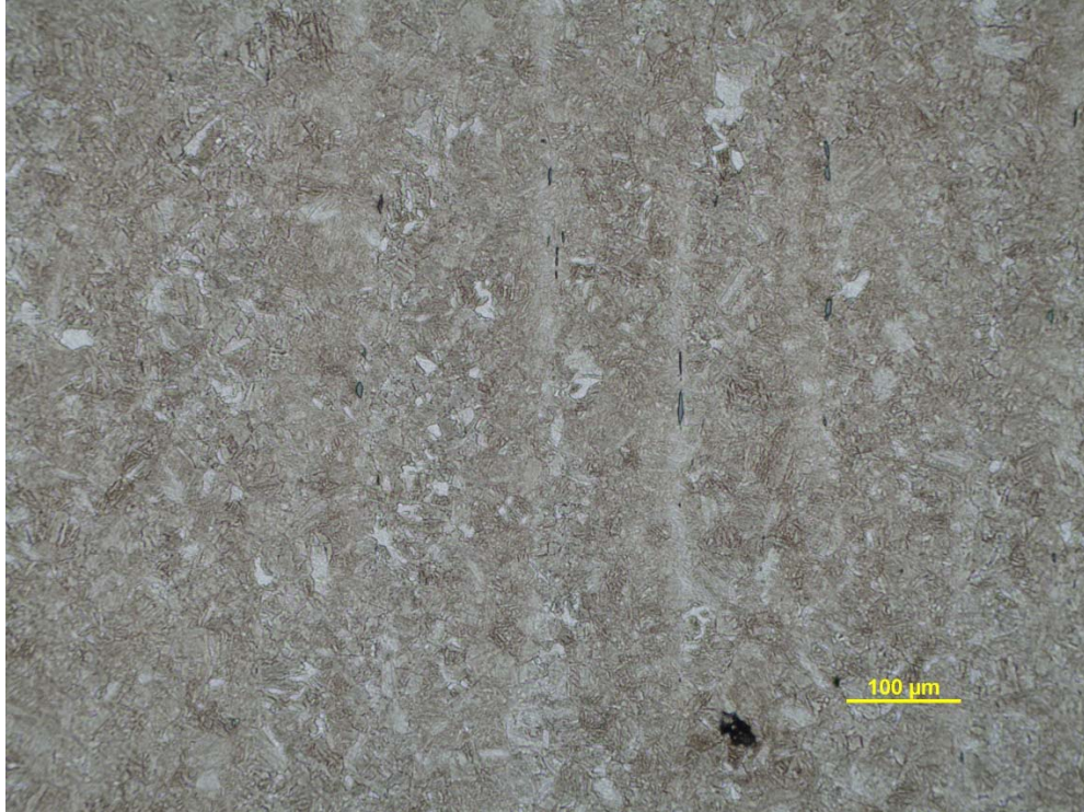
Photo 25) Another example of microstructure observed in S2-A6. Note vertical banding (alternating light-dark streaks) in grain direction. (Etchant: 2% Nital)
