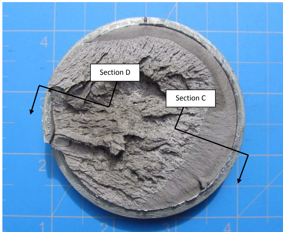
Photo 22) Fractured rod S1-G1 showing the location of cross-sections for microstructural examination and microhardness tests.
