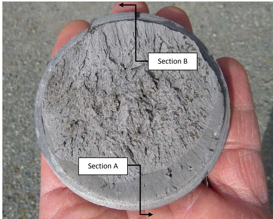
Photo 21) Fractured rod S2-A6 showing the location of cross-sections for microstructural examination and microhardness tests.
