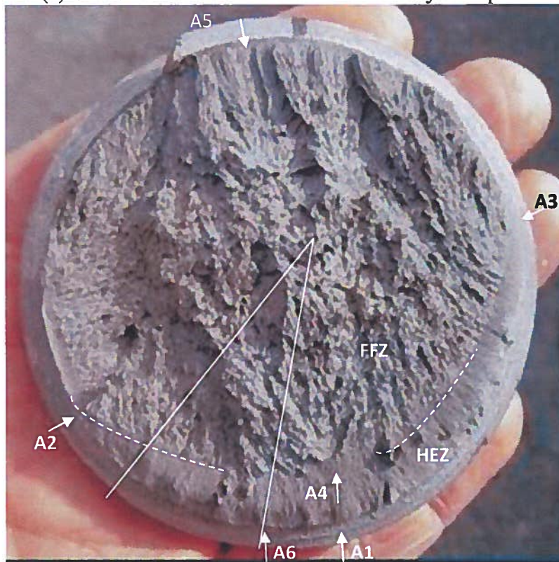
(b) Fracture face of a failed anchor rod.
