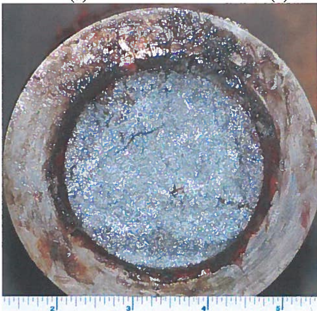
(e) Example of brittle fracture of a ductile steel
