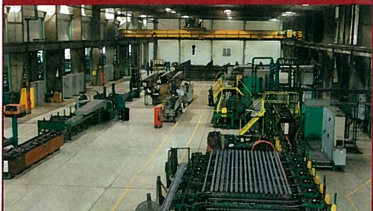
Quench and Temper production line #3.
