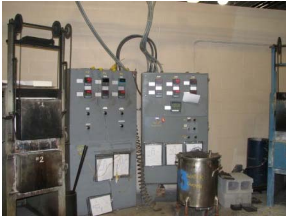
Photograph 9. When required, samples are heat-treated in calibrated ovens
