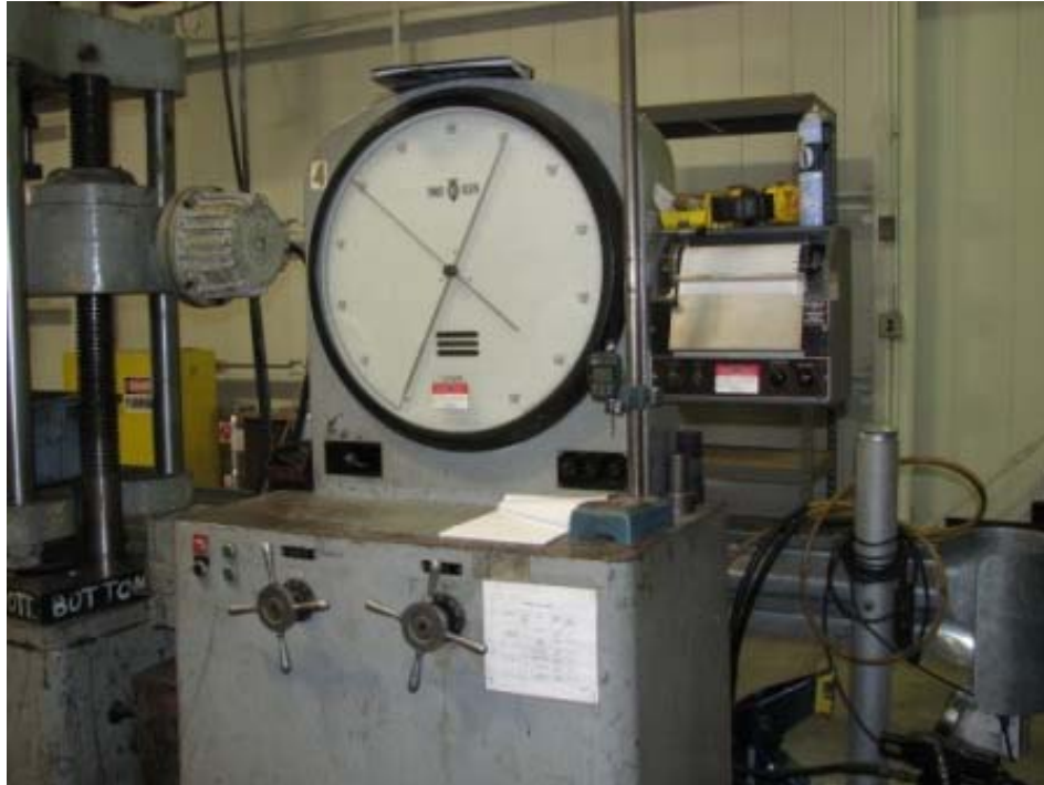
Photograph 13. Tinius-Olsen mechanical (non-computerized) tensile testing machine at TTML. Most of TTML's machines are of this type.
