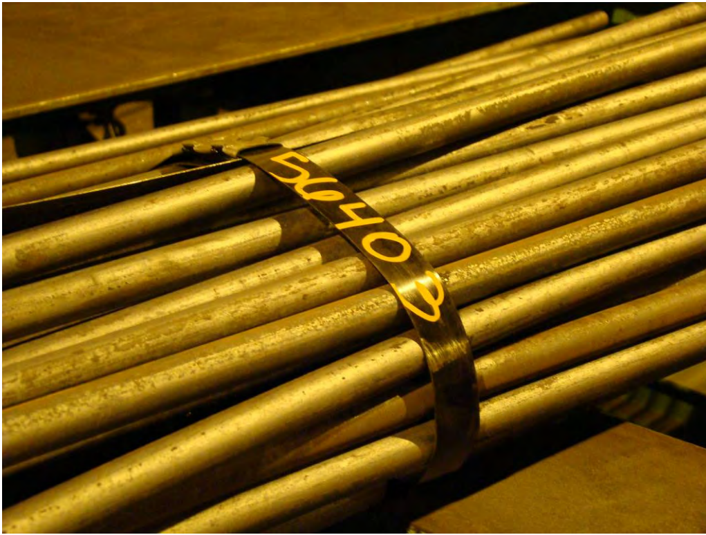
Photograph 7: Heat numbers marked on metals straps of each bundle
