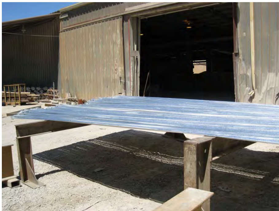
Photo 7. Components are placed on supports after hot-dip galvanizing.
