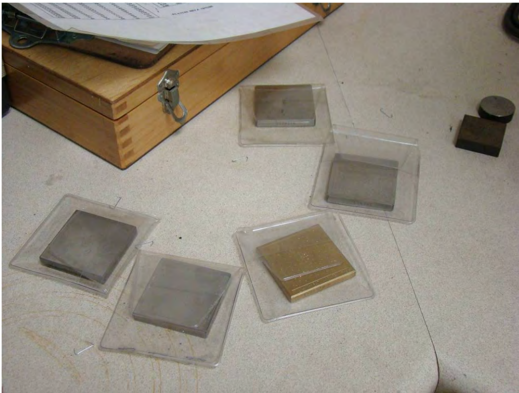
Photograph 18: Standard blocks for hardness tester verification
