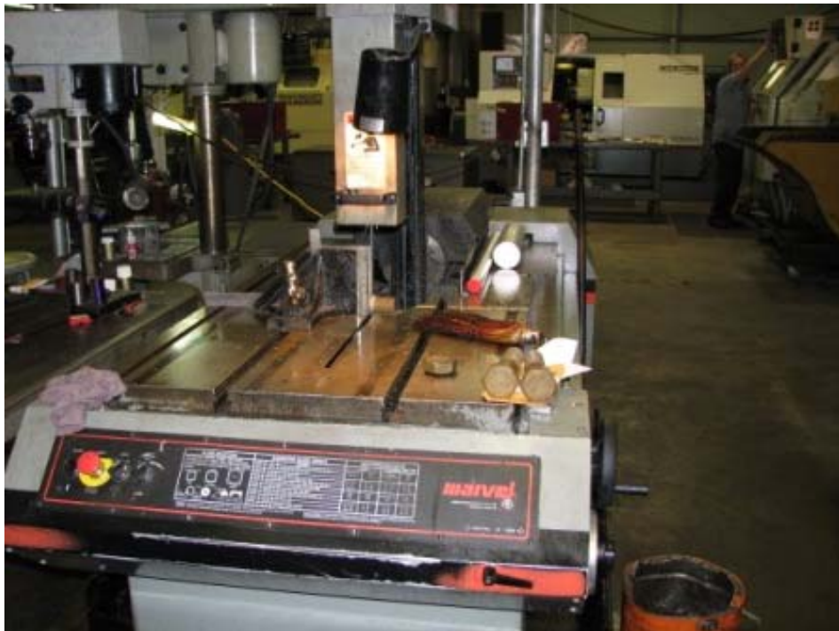
Photograph 6. Band saws in the machining area prepare samples for testing.
