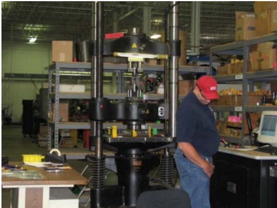
Photograph 12. The computerized tensile testing machine destructively tests a machined sample at TTML.
