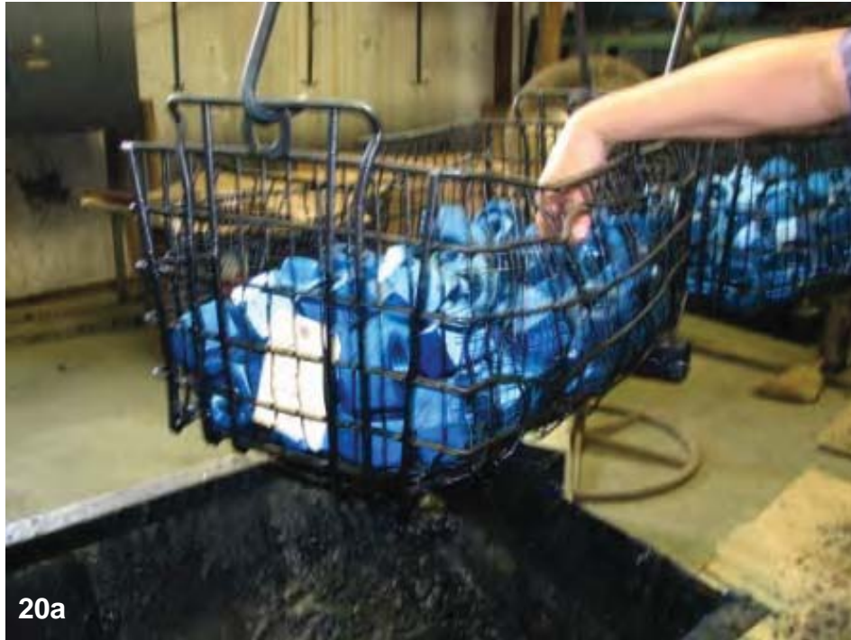
Picture 20a. The Dyson Company lubricates most nuts by dipping them into a bath.
