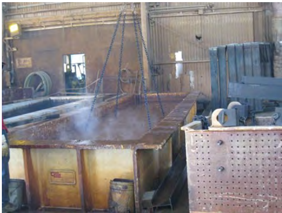
Photo 5. Components being pre-fluxed prior to hot-dip galvanizing.
