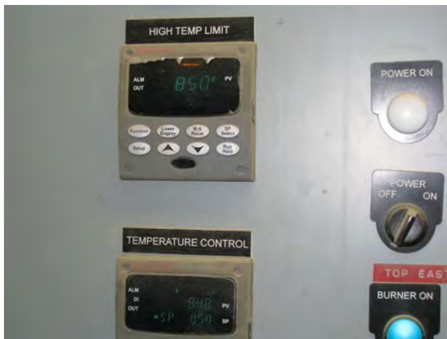
Photo 10. Automated kettle controls.
