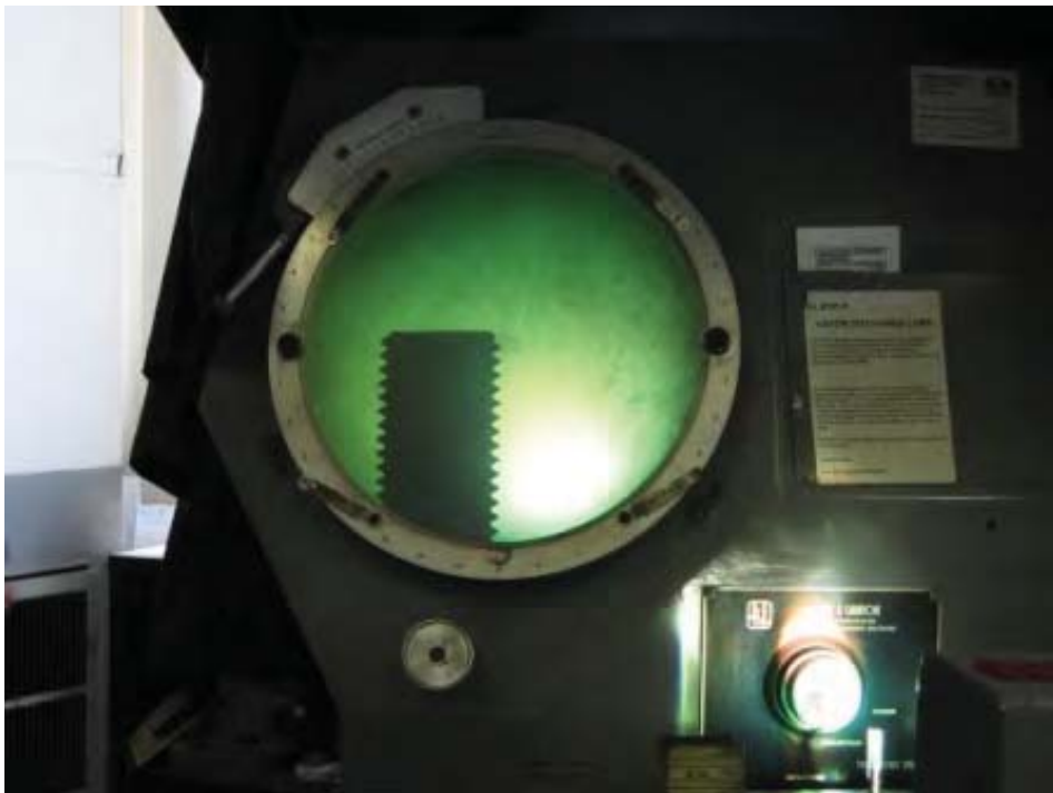
Picture 17. The Dyson Company optical comparometer displays bolt profiles for measurement.
