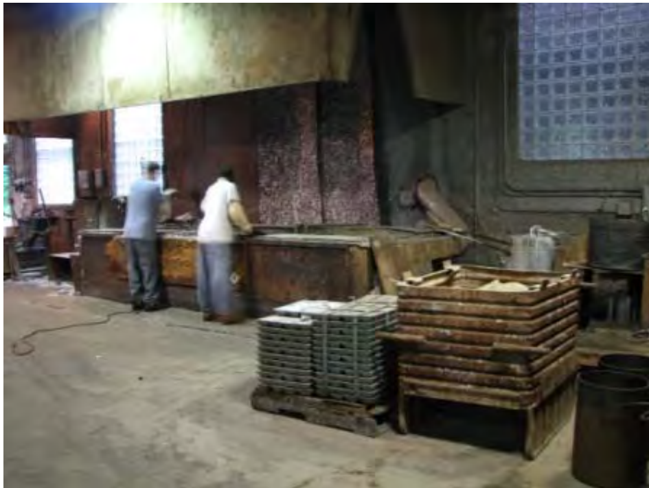
Picture 4. Hot dip galvanizing at Art Galvanizing Works is nominally time-controlled, but no clock is visible from the galvanizing line.
