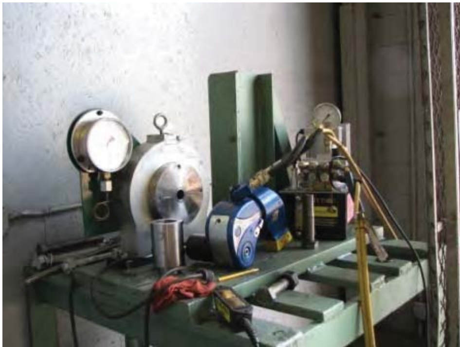
Picture 19. The Dyson Company Skidmore rocap testing machine may soon be replaced by a computerized, automated version.
