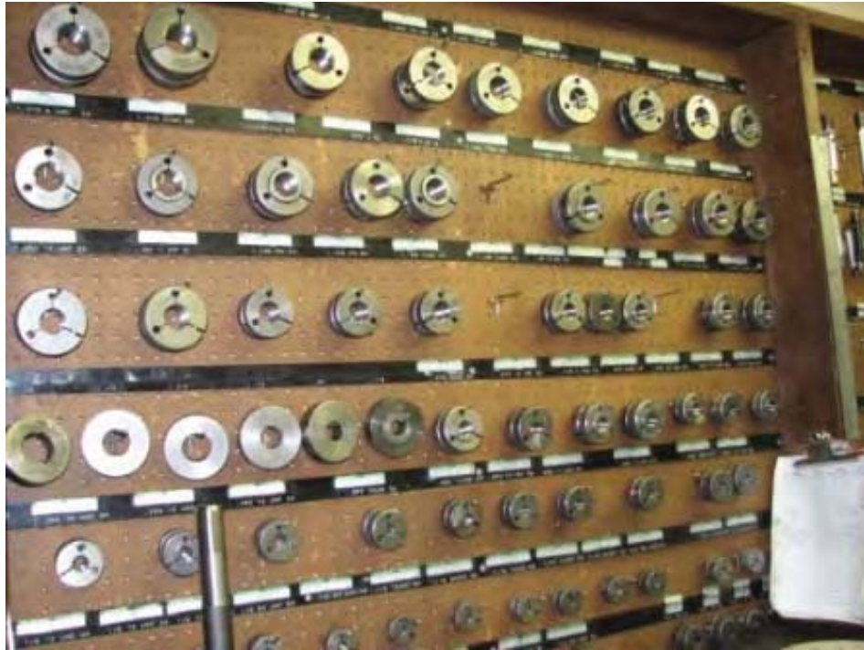
Picture 16. Dyson Company "go/no-go" gauges hang in the inspection office.
