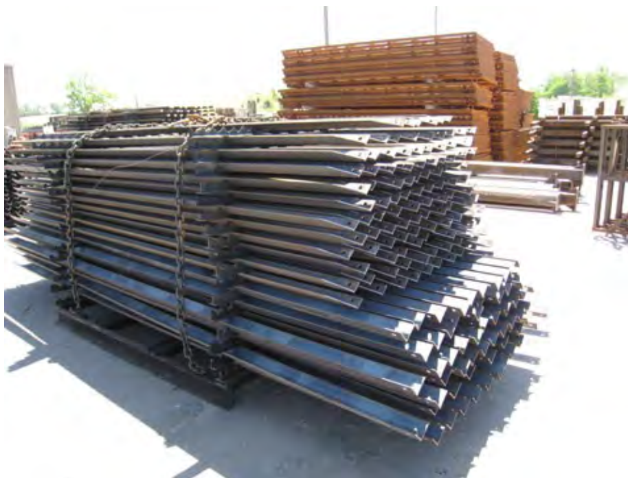
Photo 3. Galvanized components stored in the Monnig Industries yard. Material is supported by pallets, skids, and hoists while being transported by forklifts and gantry cranes through the facility.
