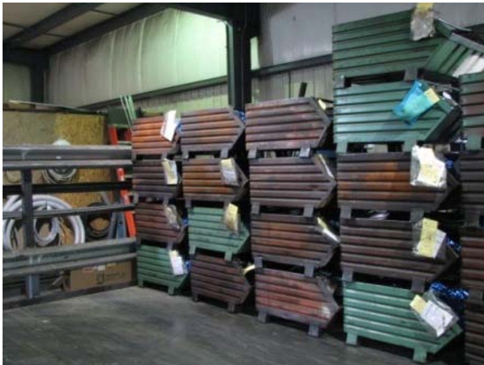
Photograph 6. Fasteners that have been galvanized and inspected numerous times, approved and ready to ship.
