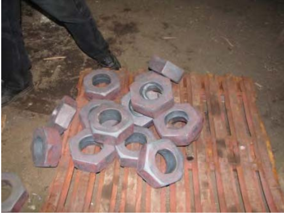
Picture 9a. One of Dyson's specialties is large forged nuts.
