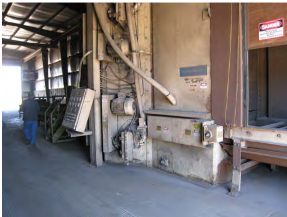
Photo 1. Automated control dry-grit blaster operated by Phoenix Industries in Unit 5.
