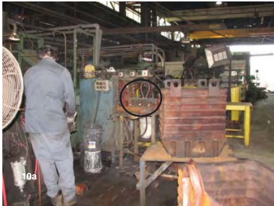
Picture 10a. A worker produces A 325 high-strength bolts at Dyson Company. Note the shaft heating oven (circled). After the shaft reaches the necessary temperature, the worker manually holds each shaft in a press, where a hex head is attached to the shaft.
