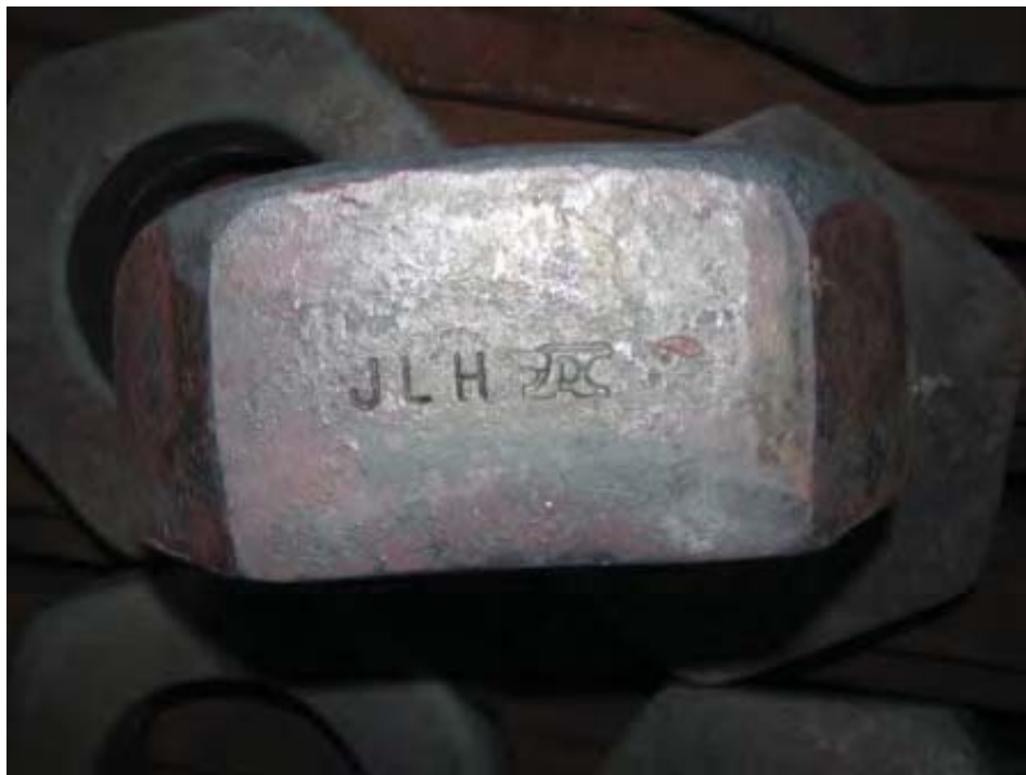
Picture 9b. Closeup of a large forged nut shows the unique three-letter job identifier and The Dyson marking. Heat numbers are added after heat treatment.
