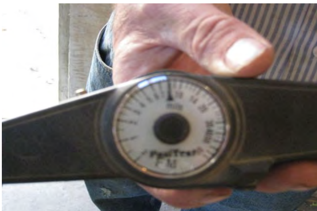
Photo 8. Mechanical mill thickness gage used by Monnig Industries to measure galvanizing thickness on components.
