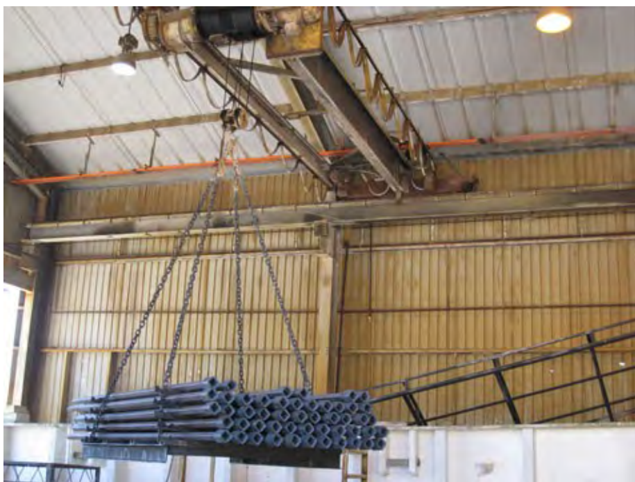
Photo 4. A gantry crane transports components to the pickling area in one of the galvanizing units.
