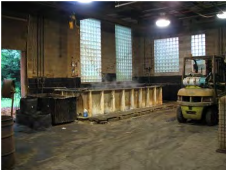
Picture 2. The acid pickling bath at Art Galvanizing Works can accommodate components up to 15 feet long.
