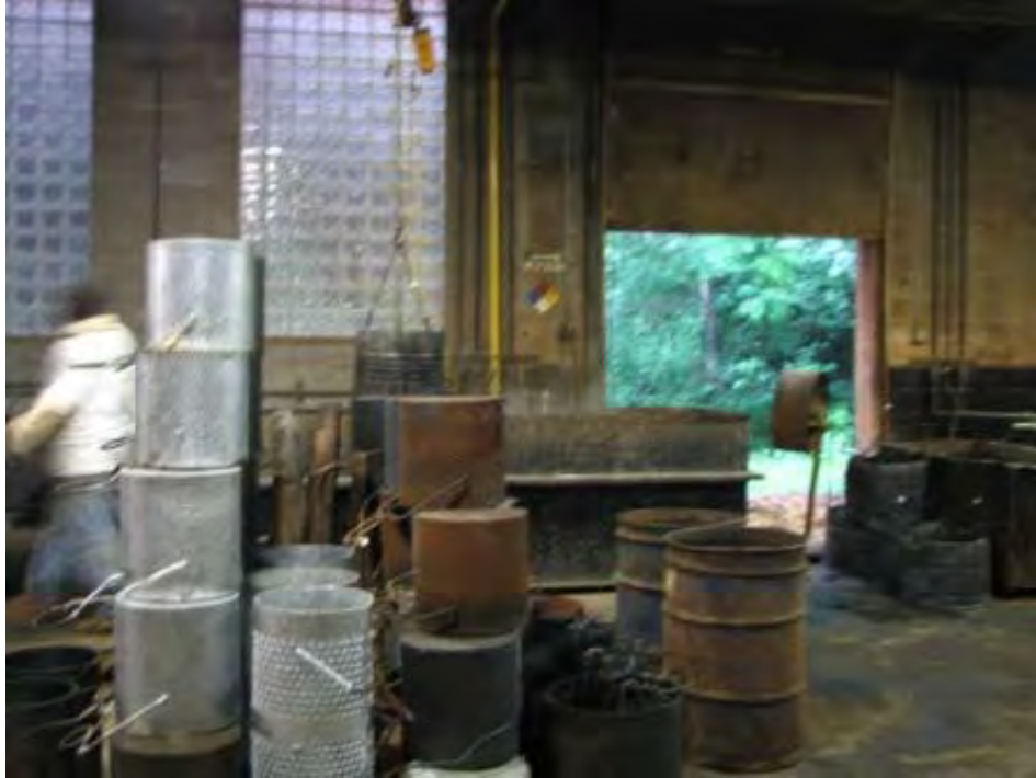
Picture 3. Components are usually small, and hot-dipped in the buckets shown, up to 3 buckets at once.
