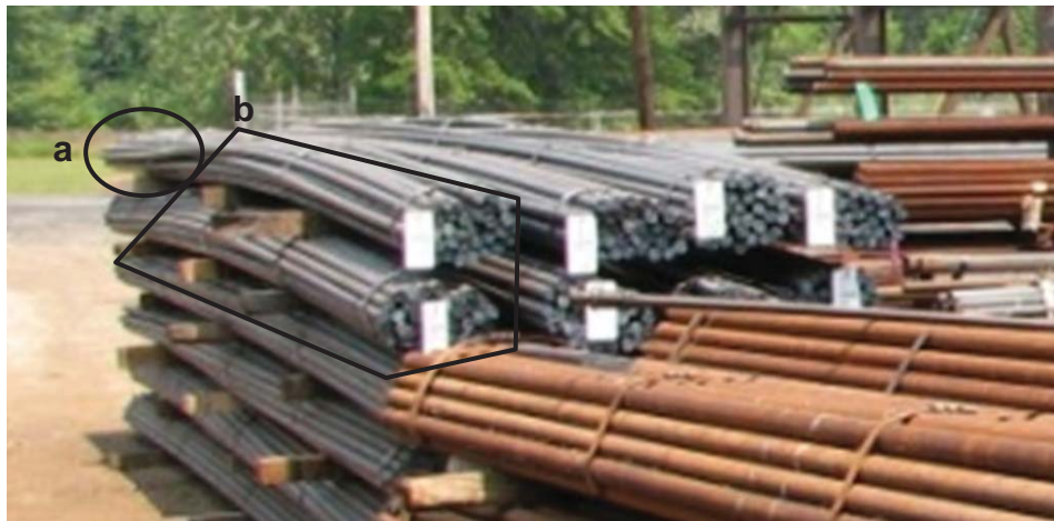
Picture 6. Closeup of the Dyson Storage Yard shows twisted (a) and bent (b) rod stock.
