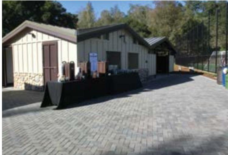
*Porous pavers in Los Gatos soften hardscapes so runoff from rain and storms can percolate into the ground, rather than pooling in surrounding residential areas.*
