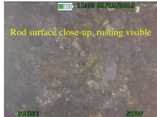
Figure 11: S2-A6 borescope snapshot
