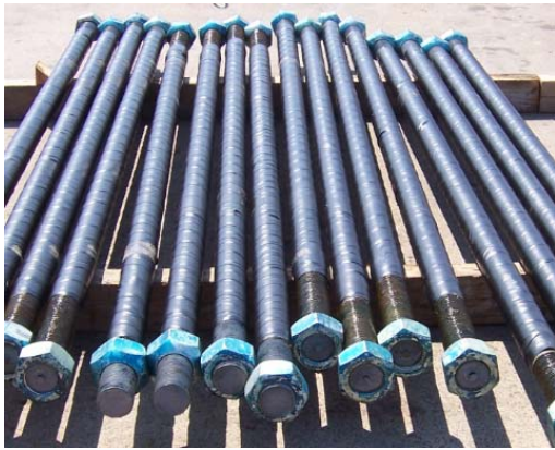
Figure 8A: Rods wrapped with Denso Tape
