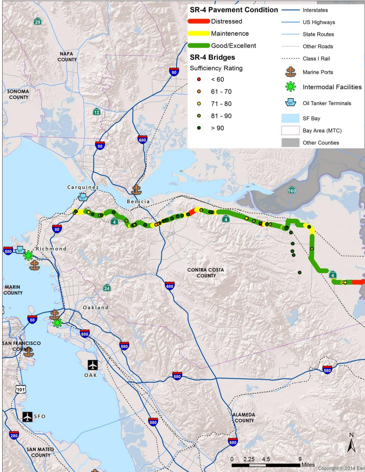
Figure 2.70 Pavement and Bridge Existing Conditions along SR 4
