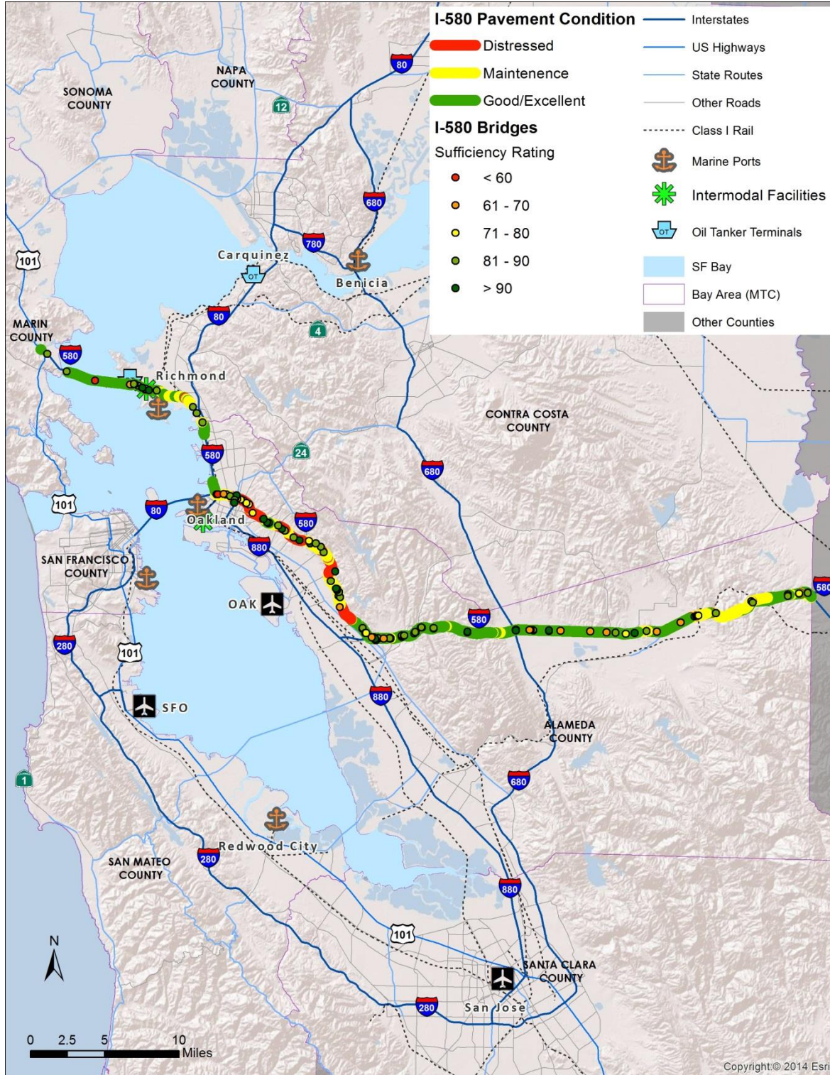
Figure 2.29 Pavement and Bridge Existing Conditions along I-580
