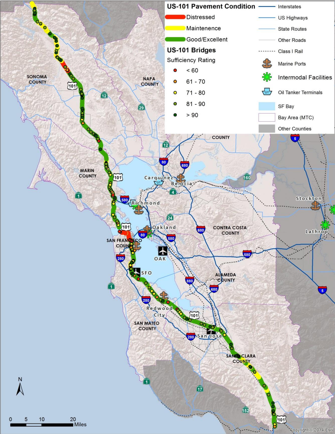
Figure 2.39 Pavement and Bridge Existing Conditions along U.S. 101
