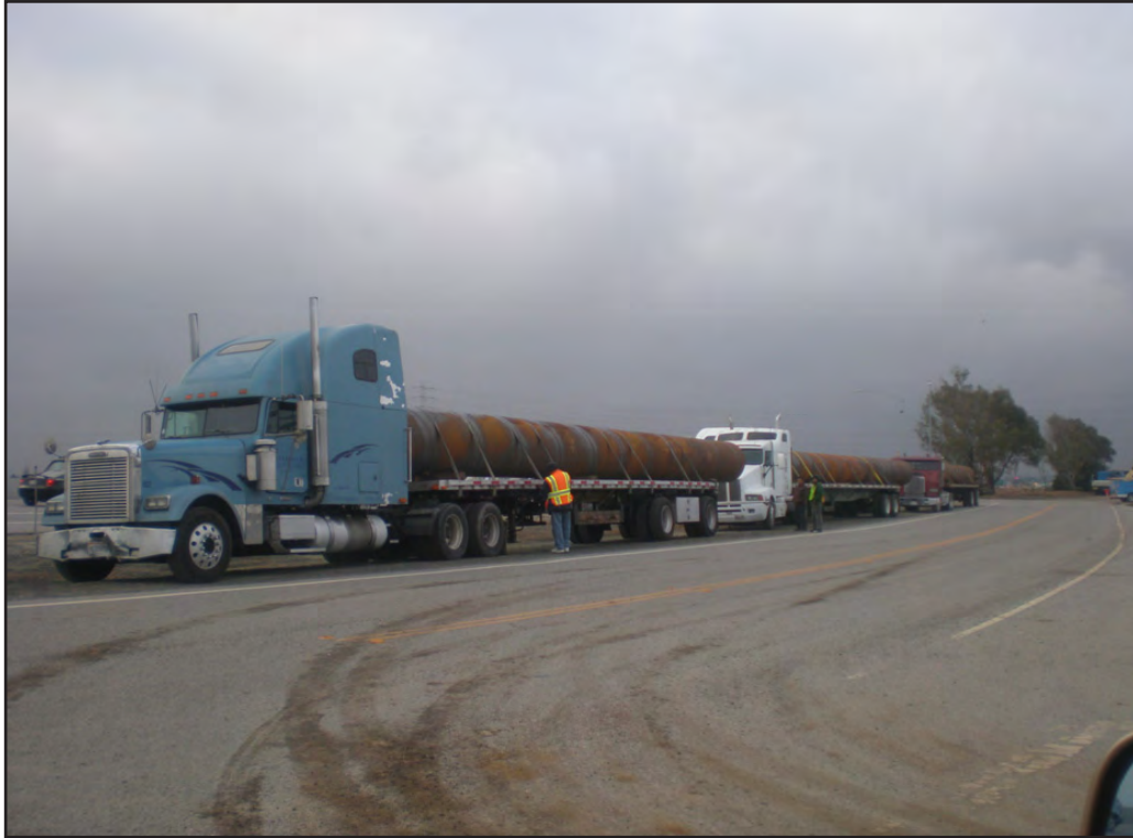
The 48-inch diameter Pipe Piles Arrive at Project Site
