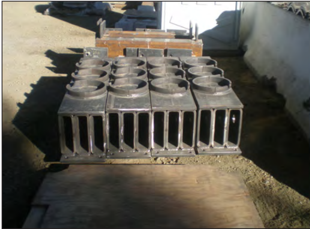
Jacks Sit within Circular Rims on top of Jacking Beams
