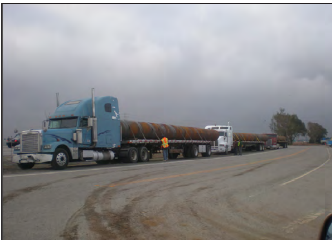
Dumbarton Bridge 48-inch Diameter Pipe Piles Arrive at Project Site
