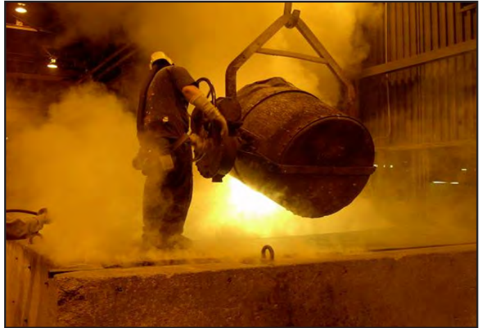
SAS Pouring for Casting for Spherical Bearings
