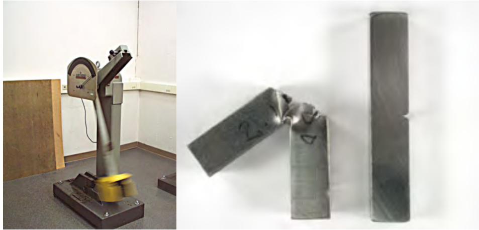
Figure 25 Charpy Toughness Test in Process (left); Tested and Untested Specimens (right)
