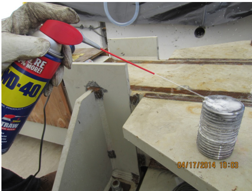
Figure 3.1-6: Fracture Preservation Operation
