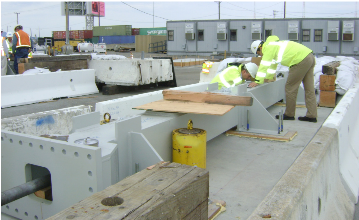
Figure 3.1-2: Test Rig for Full-Length Rods during Setup
