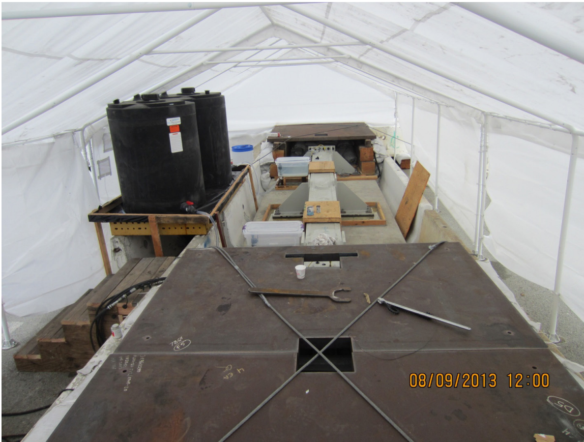
Figure 3.1-4: Test Rig after Rod Failure Showing the Effects of the Energy Released when Fracture Occurs
