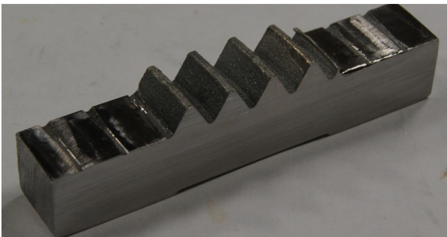
Figure 3.2-3: A Charpy-sized, Threaded Specimen for Determining KI_p
