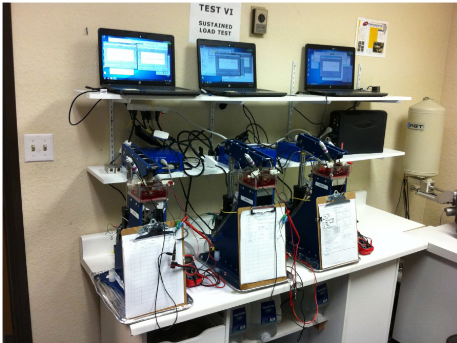
Figure 3.3-4: Three Sustained Load Test Rigs Undergoing Final Check-out Prior to Calibration
