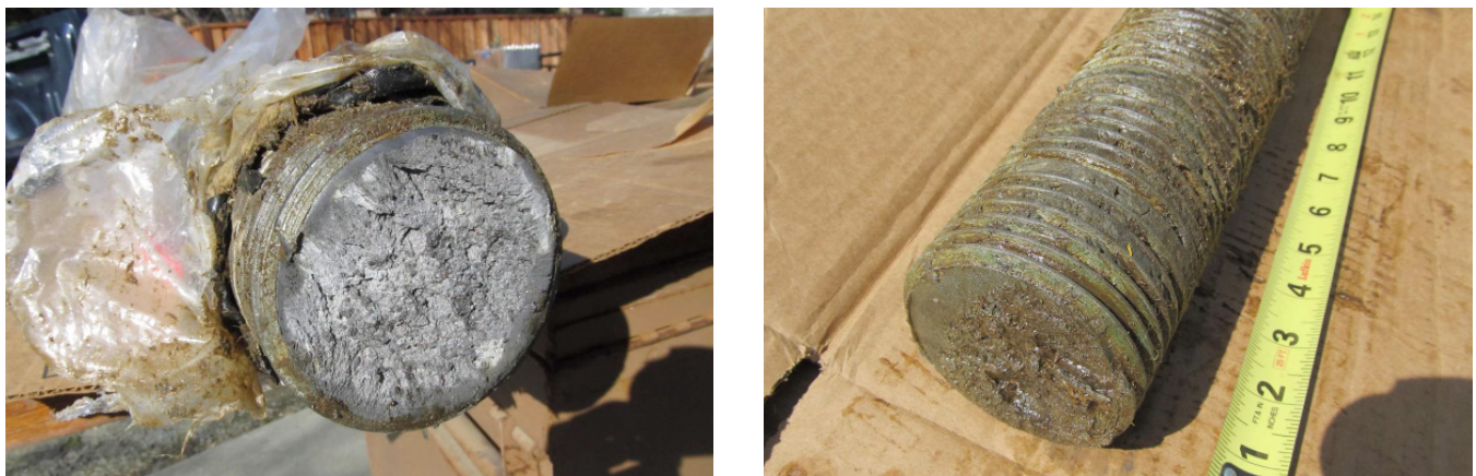
Figure 1.3-7: Pier E2 Shear Key S1/S2 Fractured Rod
