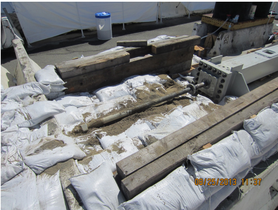
Figure 3.1-4: Test Rig after Rod Failure Showing the Effects of the Energy Released when Fracture Occurs
