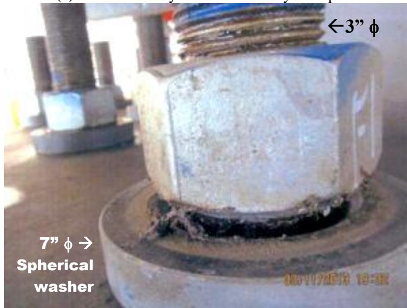
(b) A failed 3-4UNC ASTM A354 Grade BD anchor rod
